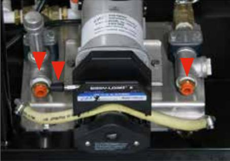
**Step 2:** Ensure the Pump Element lays on the roller and behind the clips on the Head.
