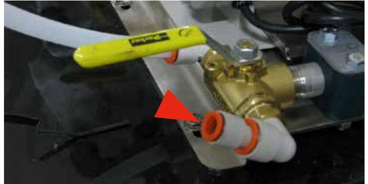
**Step 2:** Start at the bottom and insert the other end of Tubing into the Treater Chemical Inlet Assembly Press Lock Fitting.
