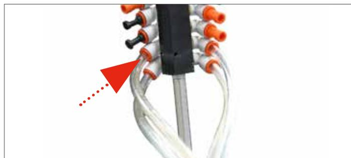
**Step 9:** Turn Pump #1 switch to the PRIME position. The pump will run, sending chemical to the chemical inlet assembly on the treater. Turn the Pump #1 switch to the OFF position.
