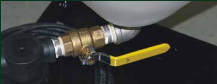
**Step 2:** Ensure the Recirculation Valve is in the TREAT mode.
