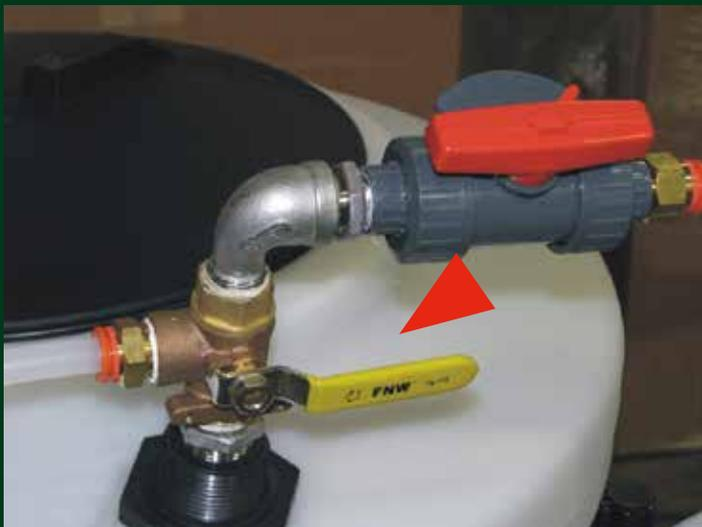
**Step 3:** Disconnect the treatment line from the Chemical Inlet on the treating head.
