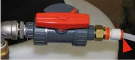
**Step 3:** Start at the bottom and insert the other end of the Tubing into the Treater Chemical Inlet Assembly Press Lock Fitting.
