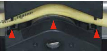
**Step 3:** Use the Pump Head handle to close the Pump Head.
