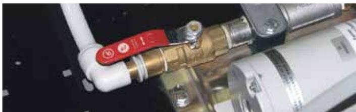
**Step 3:** Ensure the pump recirculation valve is in the RECIRCULATION mode.
