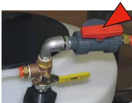
**Step 8:** Connect the treatment line into the chemical inlet assembly on the treater.
