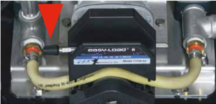
**Step 4:** Push each orange press lock fitting to release and remove the element from the pump head.
