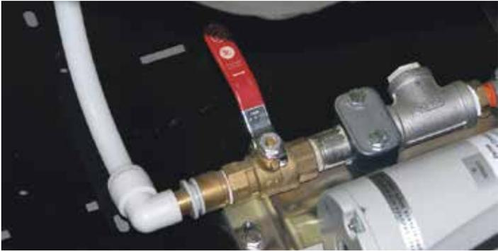
**Step 3:** Use the pump head handle to OPEN the pump head.
