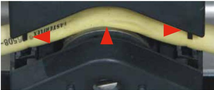
**Step 7:** Use the pump head handle to CLOSE the pump head.
