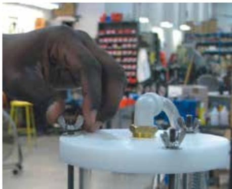
**Step 2:** Loosen the existing lower nut connected to the same stud as above.
