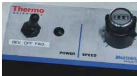
**Step 7:** Ensure the RH Basic Main Power Switch is in the ON position (UP) Power light will also indicate that the power is ON when lit.
