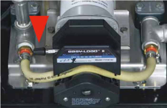
**Step 4:** Push each orange press lock fitting to release and remove the element from the pump head.
