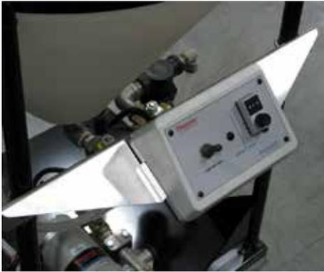
**Step 2:** Insert the U-bolt from behind the Tank Stand Frame and push through the Mount Plate. Use a 7/16" wrench and fasten in place in the following order:
