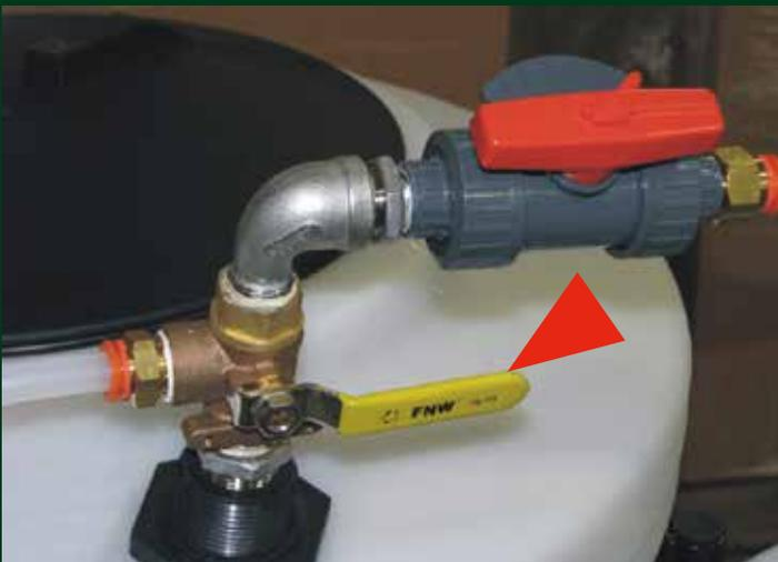
**Step 3:** Disconnect the treatment line from the Chemical Inlet Assembly on the treater.
