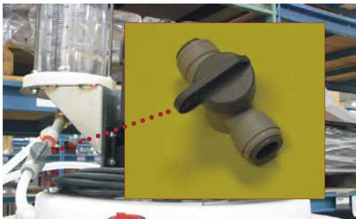
**Step 20:** When calibration is complete, turn the Recirculation Valve in the TREAT mode.
