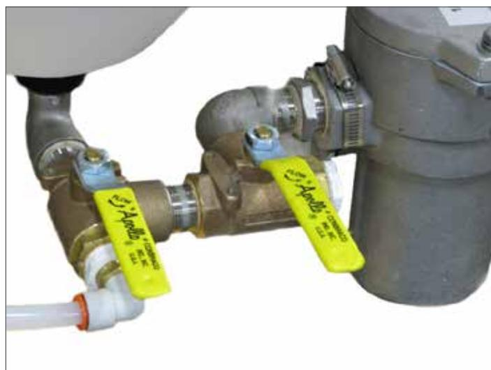
**Step 2:** Close the pump main flow valve.
