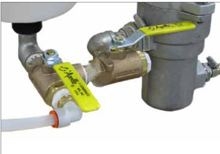
**Step 3:** Turn the pump main flow valve and recirculation Valves in the TREAT mode.
