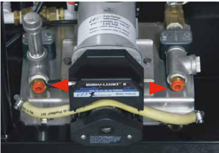
**Step 5:** Insert a new element fittings into each of the orange pump fittings.
