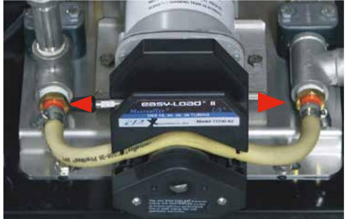
**Step 6:** Ensure the Pump Element fits properly onto the Pump Rollers and under each Clip. Failure to properly align the Element may cause Pump failure!
