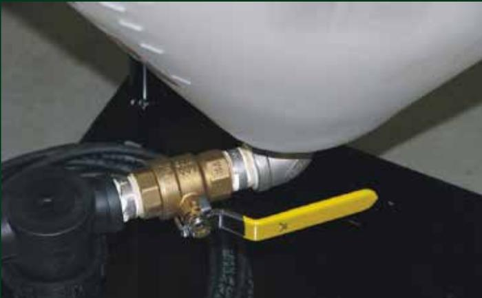
**Step 2:** Ensure the recirculation valve is in the TREAT mode.
