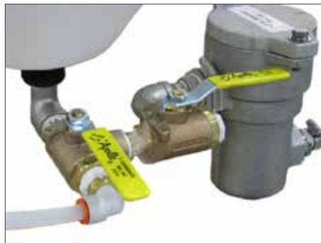
**Step 5:** Close the calibration drain valve, turn to the right.
