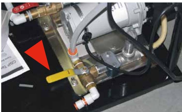
**Step 4:** Ensure the tank valves are in the TREAT mode.
