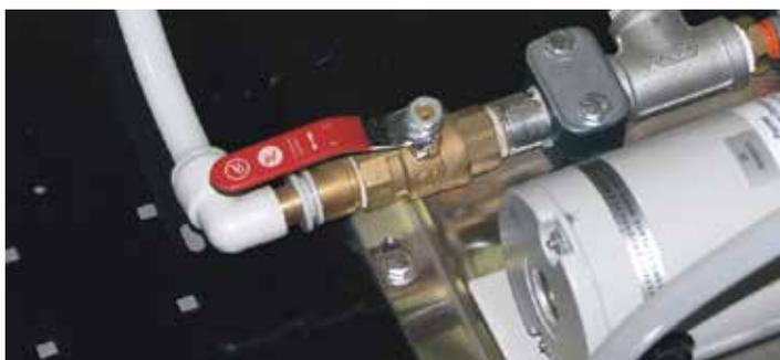
**Step 3:** Ensure the pump recirculation valve is in the RECIRCULATION mode.
