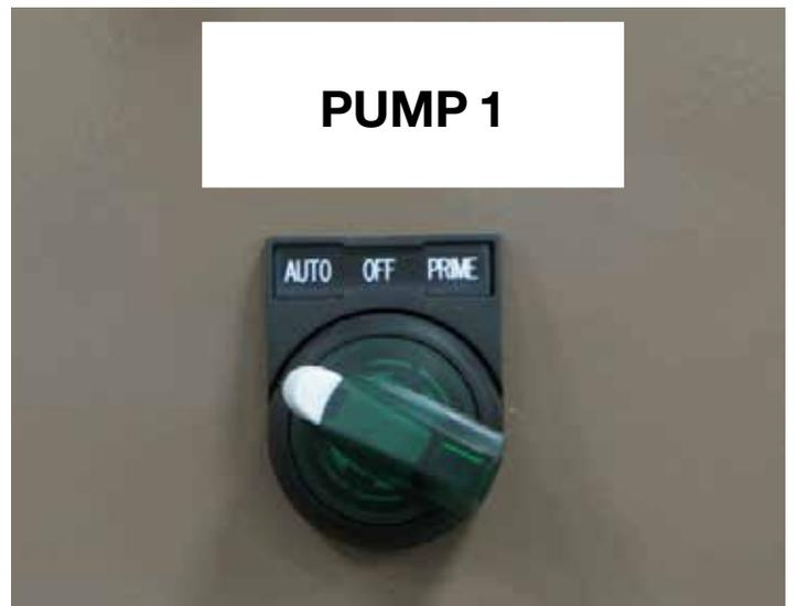
**Step 10:** Then turn PUMP #1 Switch to OFF position. Repeat this rinse process for each Pump used (1-4).
