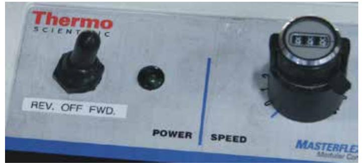
**Step 5:** Ensure the RH Basic Main Power Switch is in the ON position (UP). Power light will also indicate that the power is ON when lit.
