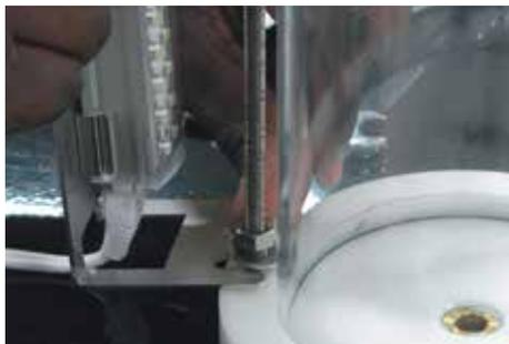
**Step 4:** Re-tighten the wing nut on the stud and the lower nut. Connect the power cord to an external 115VAC power source.
