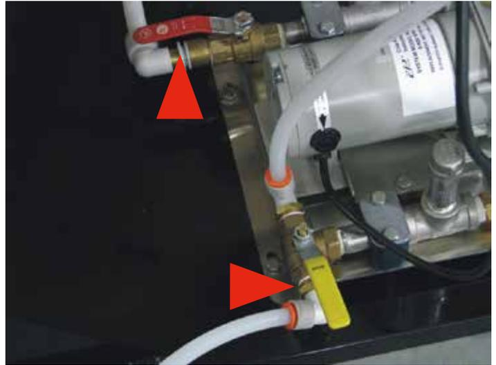
**Step 4:** Push the orange fitting and disconnect the treatment line from the Chemical Inlet Assembly on the Treating Head Assembly.
