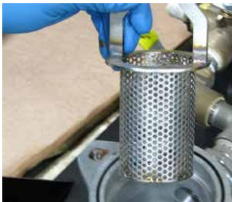
**Step 3:** Replace the filter basket in the filter body. Replace the filter cap on the filter body. Use a 9/16" wrench to tighten the two bolts.
