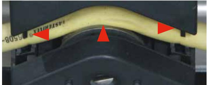
**Step 7:** Use the pump head handle to CLOSE the pump head.
