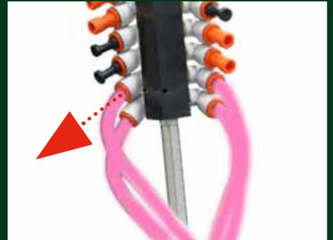
**Step 4:** Hold the treatment line in a graduated beaker (customer supplied).
