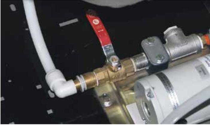
**Step 3:** Use the pump head handle to OPEN the pump head.
