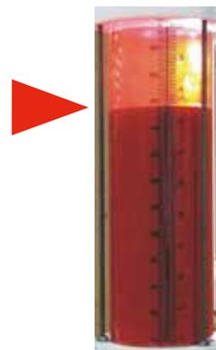
**Step 17:** Turn the RH Basic PUMP #1 Switch to OFF position. Ensure chemical does not drain from the graduated cylinder! If required, open and close the Drain Valve to ensure the Valve properly seals!
