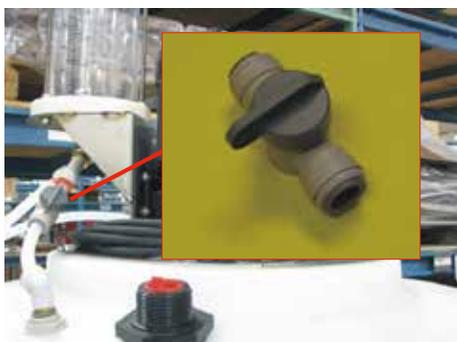
**Step 8:** Set the Pump Control to the FORWARD position.
