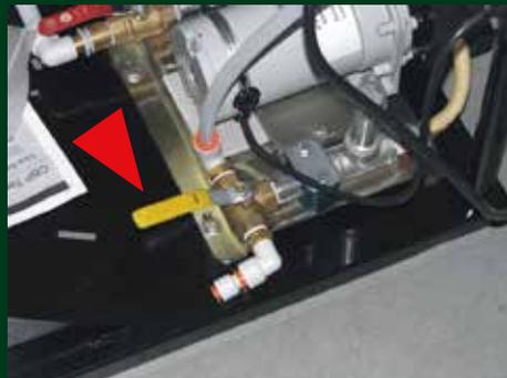
**Step 6:** Ensure the Tank Valves are in the TREAT mode.
