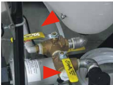
**Step 7:** Turn the Drain Valve underneath the calibration Tube to the right.
