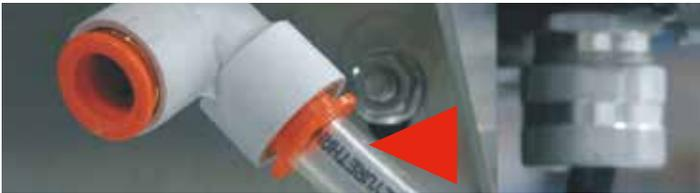
**Step 3:** Connect the Shutoff Valve to the piece of 1/2" Tubing.
