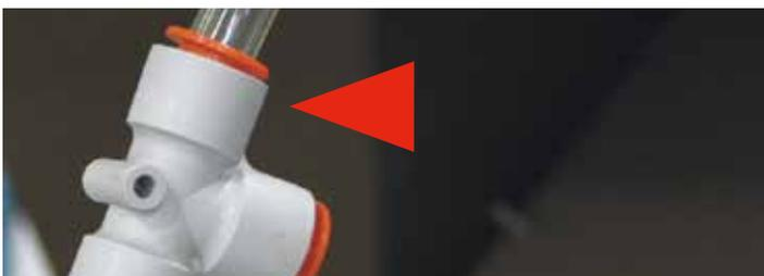
**Step 10:** Cut to fit and connect the remaining piece of Tubing to the 90° elbow press-lock fitting, located on top of the Calibration Tube.
