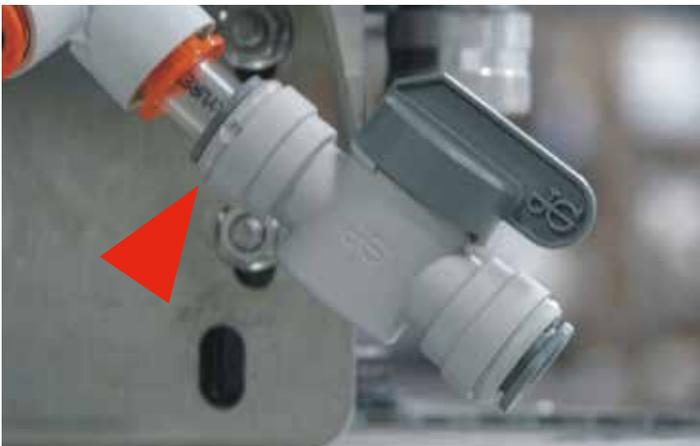
**Step 4:** Remove the Calibration Port Plug from the top of the Tank. Cut to fit a piece of the factory supplied 1/2" Tubing. Press it into the Shutoff Valve. Press the other end into the 90° Elbow Press-lock Fitting and install on top of the CBP Tank.
