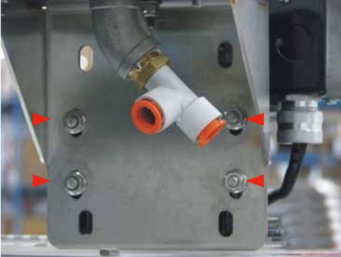
**Step 2:** Cut a 3" piece of the factory supplied 1/2" Tubing. Press it into the Male Run Tee (attached to the bottom of the Calibration Cylinder).
