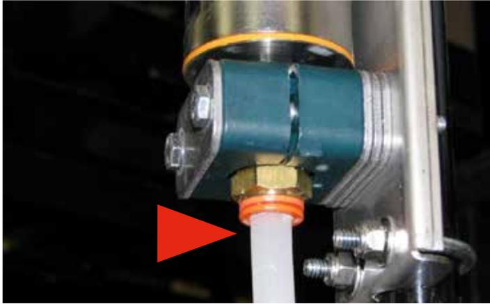
**Step 14:** Connect one end of the Treatment Tube to the Press-lock Fitting on the Flow Meter Assembly (left side).
