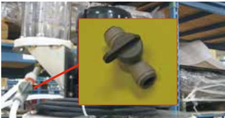
**Step 19:** When calibration is complete, turn the Recirculation Valve in the TREAT mode.
