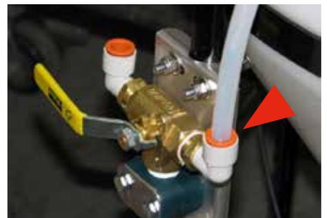
**Step 7:** Remove the second Vent Plug from the top of the CBP Tank. Cut a 2" piece of Tubing. Press it into the Vent Press-lock Fitting.
