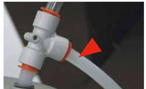
**Step 12:** Cut to fit and connect the other end of the Vent Tube to the Press-lock Fitting on the pump, located underneath the CBP Tank.
