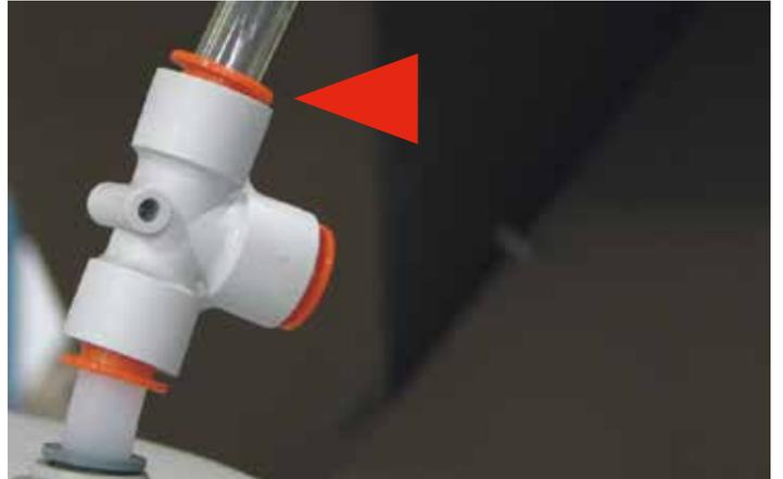
**Step 10:** Cut to fit and connect the remaining piece of Tubing to the 90° elbow press-lock fitting, located on top of the Calibration Tube.
