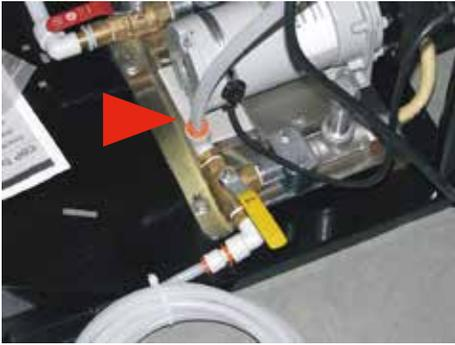
**Step 7:** Remove the second Vent Plug from the top of the CBP Tank. Cut a 2" piece of Tubing. Press it into the Vent Press-lock Fitting.
