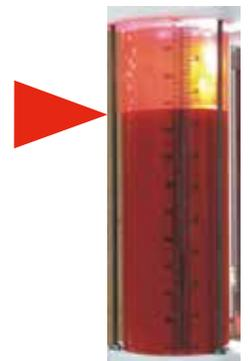
**Step 16:** Turn the RH Basic PUMP #1 Switch to OFF position. Ensure chemical does not drain from the graduated cylinder! If required, open and close the Drain Valve to ensure the Valve properly seals!
