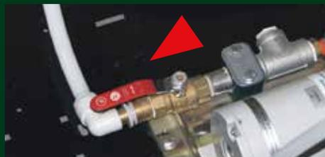
**Step 5:** Ensure the Recirculation Valve is in the recirculation mode.
