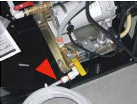
**Step 14:** Insert the other end of the Tubing into the Treater Chemical Inlet Assembly Press Lock Fitting.
