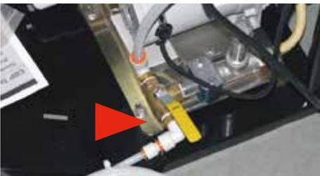
**Step 20:** Turn the RH Basic PUMP #1 Switch to the PRIME position. The Pump will run, purging the treatment lines of air and fill with chemical. Then turn PUMP #1 Switch to OFF position. Repeat for all Pumps used (1-4).
