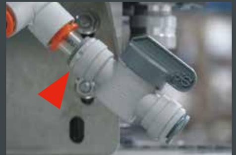
**Step 4:** Remove the Calibration Port Plug from the top of the Tank. Cut to fit a piece of the factory supplied 1/2" Tubing. Press it into the Shutoff Valve. Press the other end into the 90° Elbow Press-lock Fitting and install on top of the CBP Tank.
