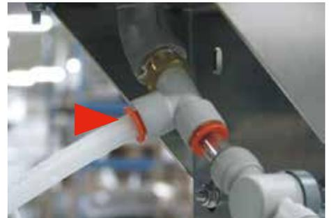
**Step 6:** Connect the other end of the Recirculation Tube to the 1/2" Press-lock Fitting on the Flow Meter Assembly (right side).
