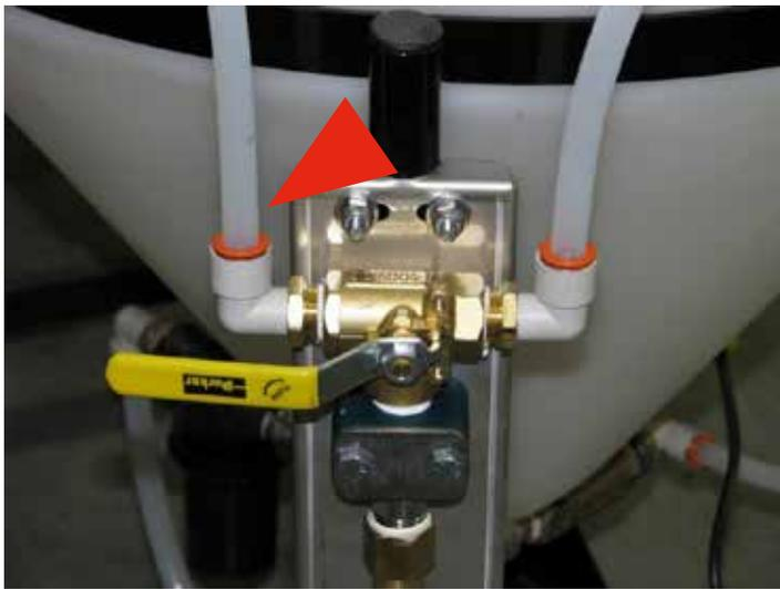
**Step 15:** Insert the other end of the Tubing into the Treater Chemical Inlet Assembly Press Lock Fitting.
