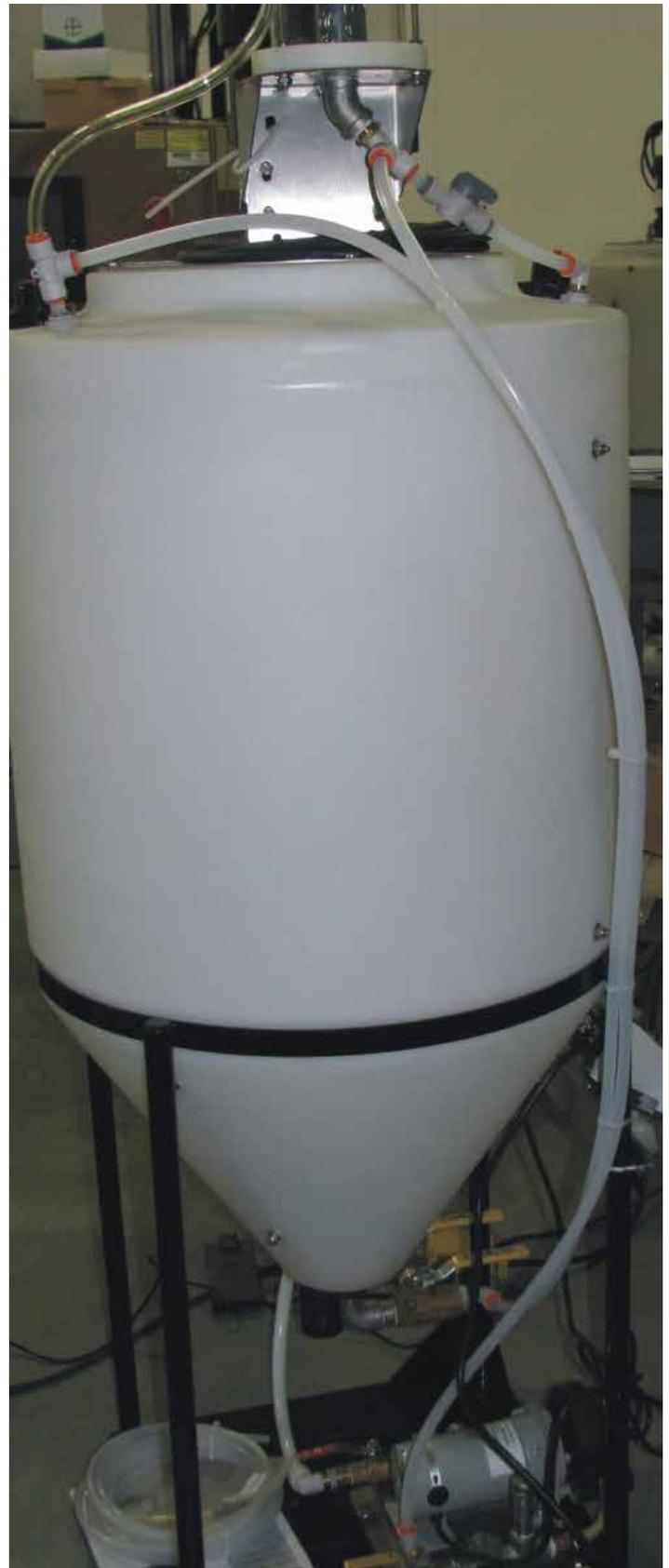
Top Calibration installed without a Flow Meter
