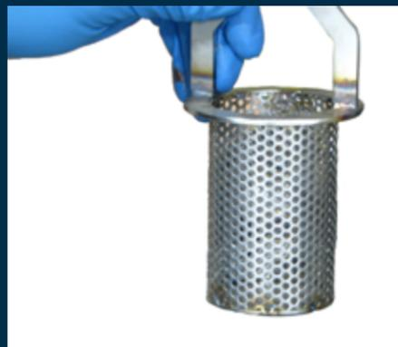
**Step 4:** Replace the filter basket in the filter body. Replace the filter cap on the filter body. Use a 9/16" wrench to tighten the two bolts.
