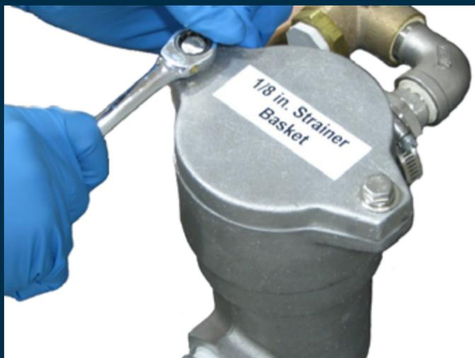
**Step 3:** Remove the filter screen from the filter bottom and check it for clogging and material build-up. Clean it thoroughly.
