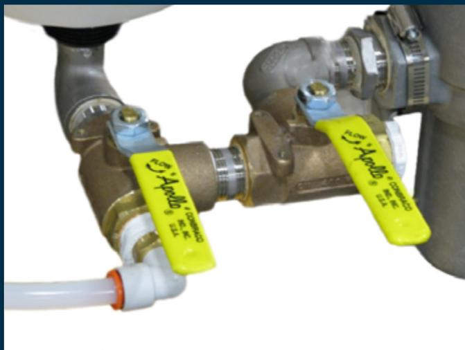
**Step 2:** Check filters periodically for clogging issues. Use a 9/16" wrench to remove the filter cap from the filter body. Remove the filter basket and clean thoroughly.
