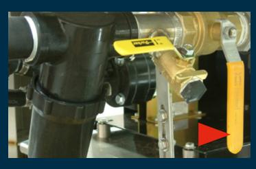
**Step 2:** Remove the retaining U-clips from both the top and bottom hoses connected to the D3 Pump. Release the clips, unscrew and remove both couplers (chemical **IN** and **OUT**) from the Pump.
