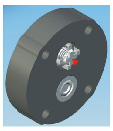
Step 15: Remove the Screw, O-ring and Follower from the center of the Diaphragm. Remove the Diaphragm from the Diaphragm Plate and inspect it carefully. A ruptured or torn diaphragm generally indicates a pumping problem. Replacing the diaphragm is absolutely necessary if a ruptured, torn or severely worn diaphragm is found. Remove the Diaphragm Plate only if it needs to be replaced due to excessive wear or damage!
