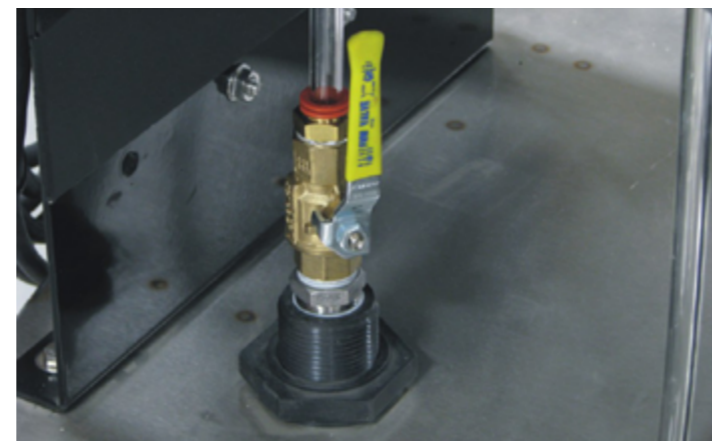
Calibration Valve in Treat Mode drains Graduated Cylinder
