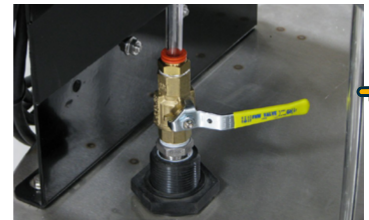
Calibration Valve in Calibration Mode fills Graduated Cylinder
