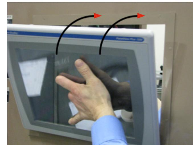
**Step 6:** Hold the HMI in place with one hand and fasten it to the control panel (backside) with the supplied eight (8) fasteners (see inset photos below). Use a Phillips screwdriver to tighten snug each fastener to the control panel door.
