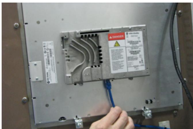
**Step 7:** Cut off the existing control panel power cord receptacle. Strip leads back and connect them to the plug provided with the touch screen. Insert the plug into bottom of the HMI. Tighten two screws.
